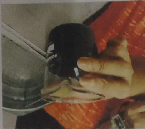
Figure 6. Dispersion of MW-CNT on ultrasonication bath
