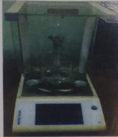
Figure 15. Mettler Toledo analytical balance with a density measurement kit.
