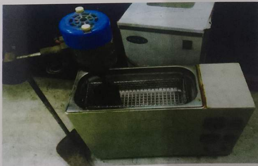
Figure 7. Visco jet stirring is going on with simultaneous ultrasonication
