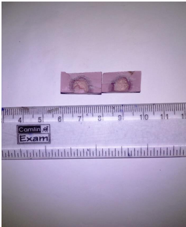
Fig-18: Corroded of Cr 10 (O) sintered at 1450°C Fig-19: Corroded of Cr 10 (R)
