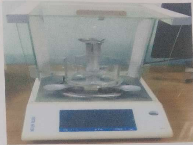
Figure 12. Mettler Toledo analytical balance with a density measurement kit.
