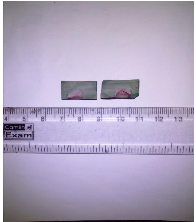
Fig-18: Corroded of Cr 10 (O) sintered at 1450°C Fig-19: Corroded of Cr 10 (R)
