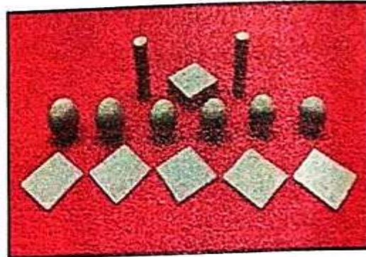
Fig.10: Photographs of the laboratory made different component using IREL made 9mole % MgO stabilized zirconia powders.
